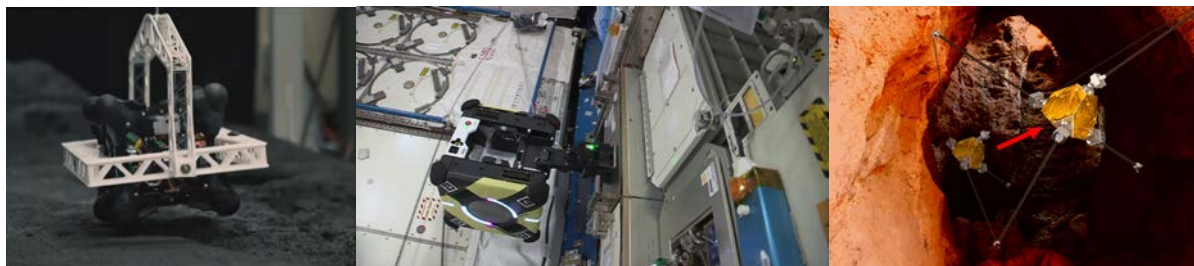
Box 3. The development of rovers for the exploration of small Solar system bodies required the development of a one-of-its-kind 6 DoF microgravity test bed built on a powered gantry crane; the gimbal frame allows the robot to rotate in all three axes (left). Robotic grippers and guidance algorithms for satellite servicing are currently being tested on the
