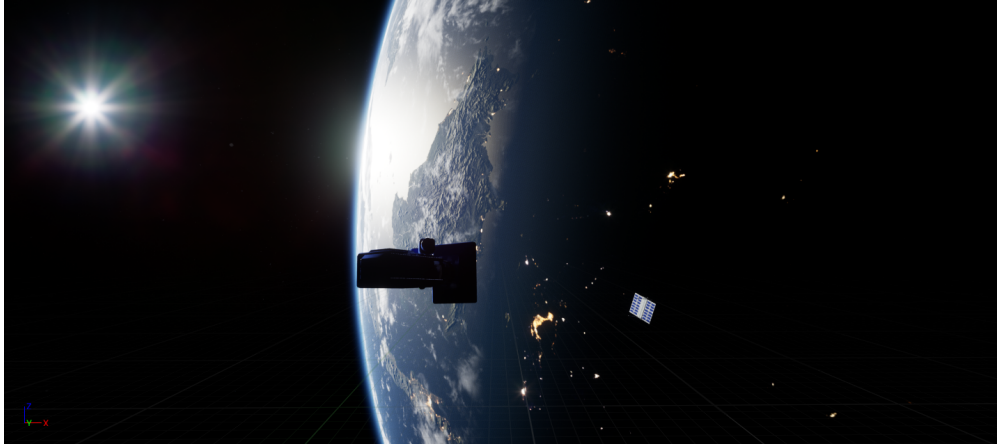
Fig. 7 The UE editor view of the scene. The scene consists of the camera, a CubeSat target, Earth and the Sun. Figure from Ahmed et al. [6]
